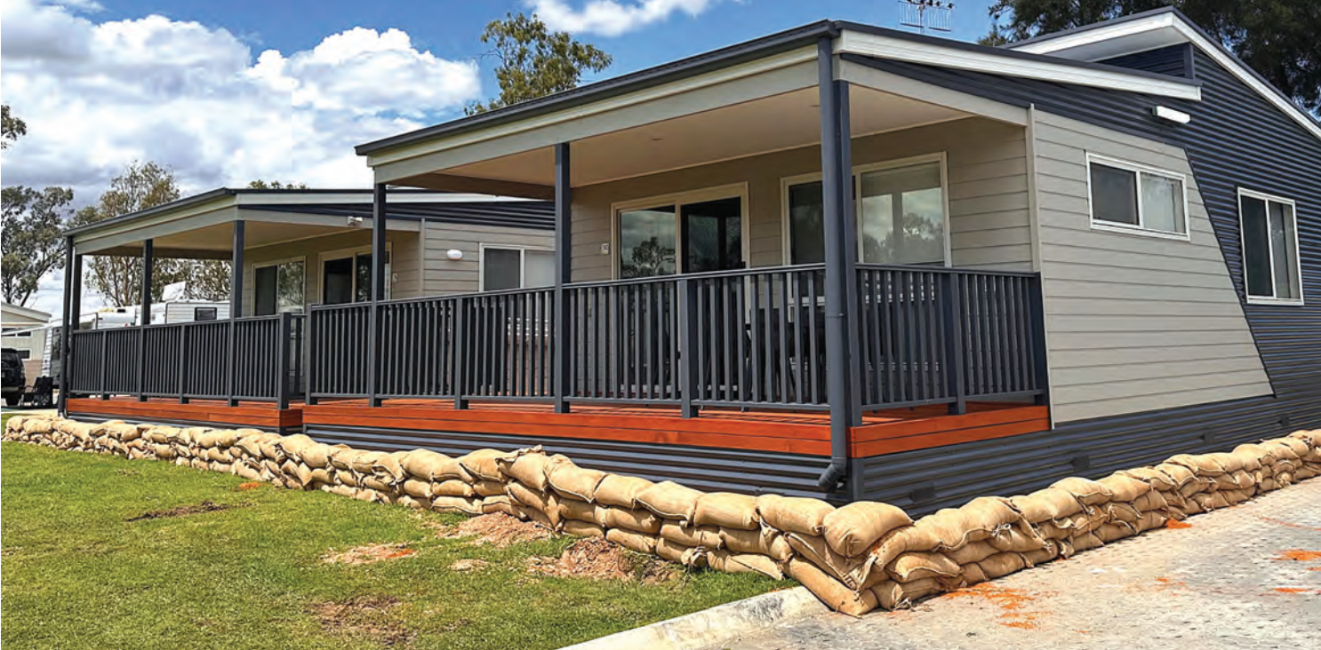
A 2.4-metre high levee stretching 300-metres has protected the Waikerie Holiday Park from the River Murray flood, which peaked at Waikerie last week. PHOTO: supplied
